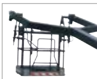
Pendular platform allows work under-bridges
