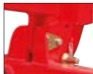
Foldable tines: suitable for road traffic
